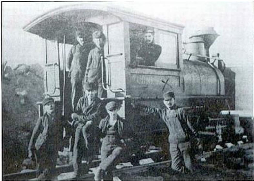
At one time, the Harbison-Walker Refractories Company fielded quite a roster of these 3-foot gauge O-4-OT dinkeys to trundle ganister rock from its extensive quarry on Jack's Mountain, across the Juniata River, to its silica brick plant at Mount Union. Obtaining any definitive data on these diminutive locomotives at this late date would be a formidable task. — Mount Union Area Historical Society
